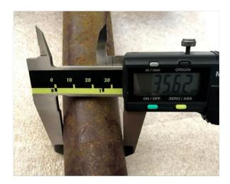
The rusted pipe has a tapered width. Below is an image to show the width of the pipe (~35.6mm)
