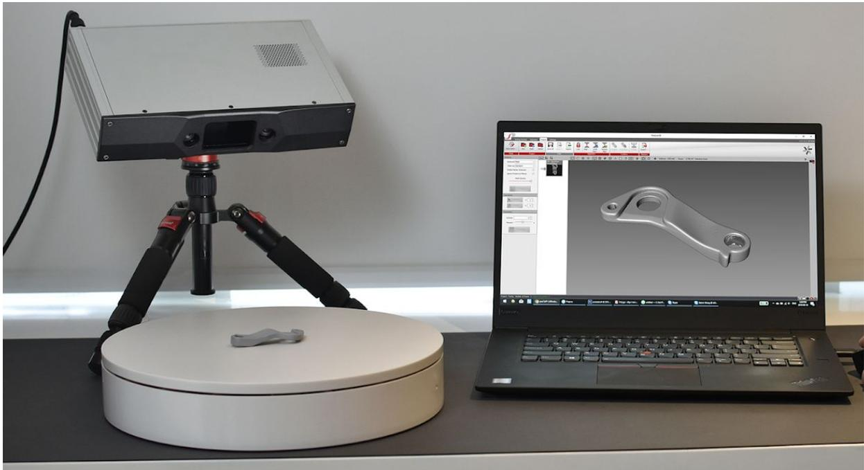
Go to the **Project** tab in FlexScan3D and you should be able to see the object in the live feed camera window on the bottom right of the screen. In order to get the correct camera focus, adjust the distance between the scanner and the object so that the red crosshairs in both the cameras intersect at the same point on the object as shown in the screenshot. You can set to projector pattern to **FOCUS** and align the red crosshairs over the main center focus pattern crosshair.
