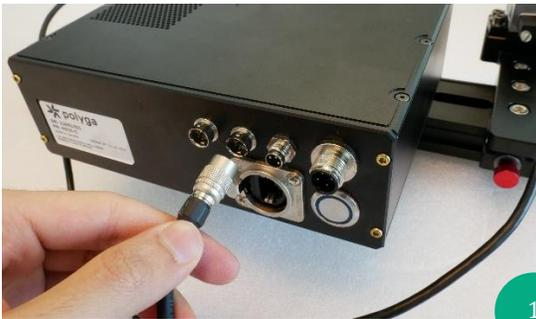
Attach the first trigger cable
