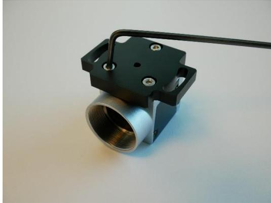
3. Attach the mounting plate on top of the camera slider using the 3x mounting screws(M4).
