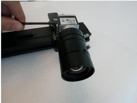
5. Attach the camera lenses on the cameras using the threads as shown below.
