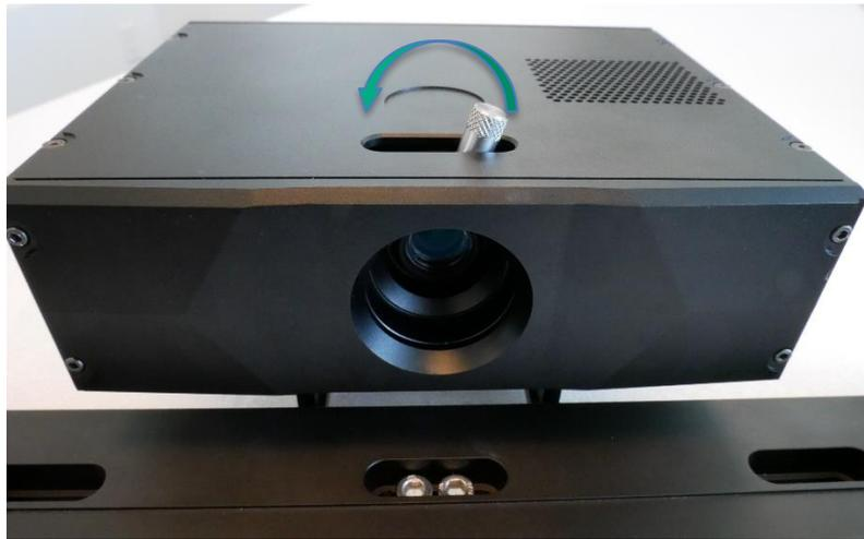
4. After adjusting the projector focus, adjust the camera position, focus and exposure.
