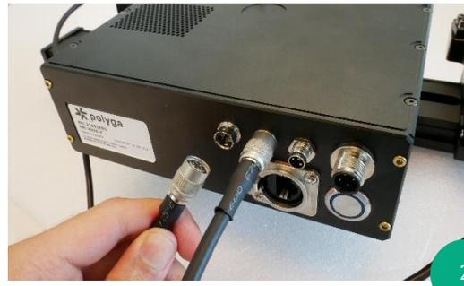
Attach the second trigger cable
