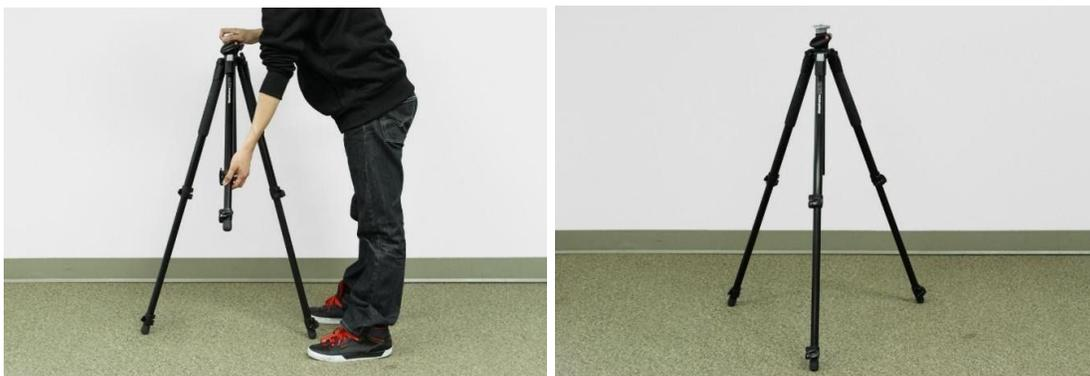
Attach the tripod head to the legs by firmly twisting the tripod head until it is hand tight. (Some scanners will arrive with the tripod head already attached.)
