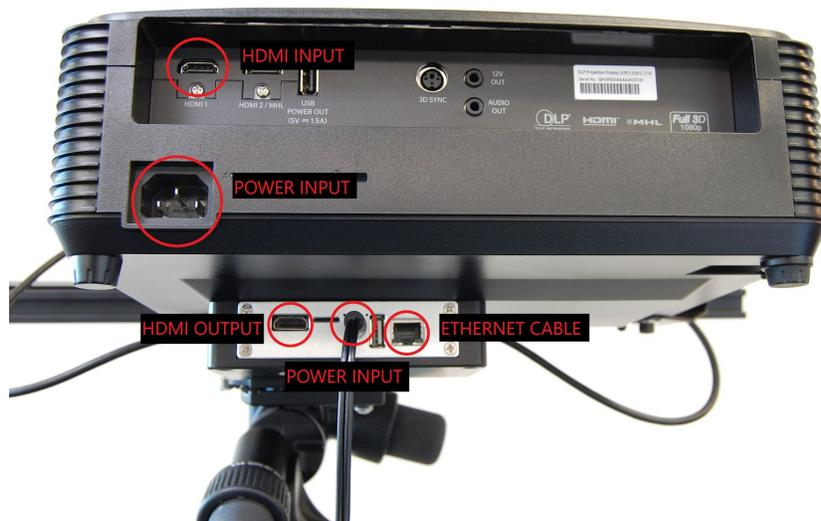
Next, Plug in the power cord into the power inlet for the Projector.
