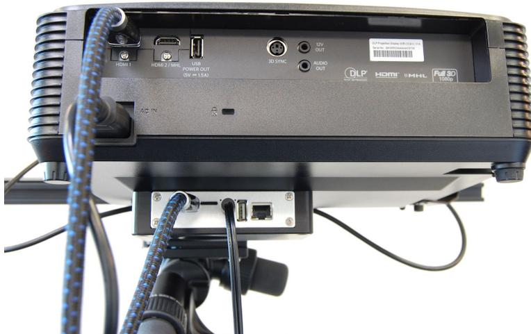
Finally, connect the RJ45 cable to the ethernet port in the Trigger Box. Connect the other end to the ethernet port of your PC on which you intend to use the 3D Scanner.
