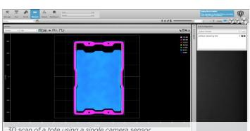
3D scan of a tote using a single camera sensor
